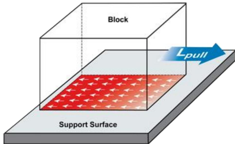
**Friction** is the force which develops at an interface resisting sliding of one surface relative to the other
